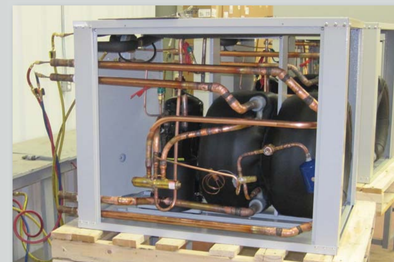
Copper is used extensively in DX units.
