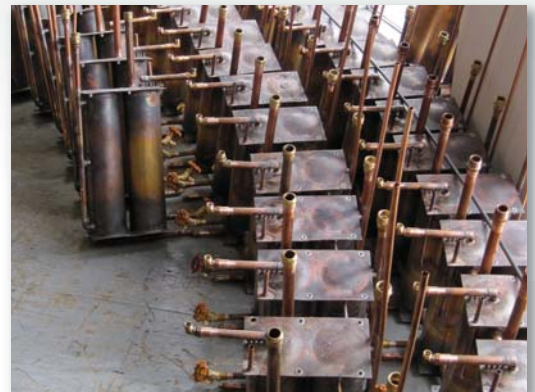
Copper solar heat exchanger units fabricated for Solar City in Halifax N.S. Photo: R.J. Catterall.
